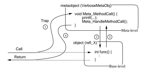
Figure 1: Metaobject protocol of Open C++
