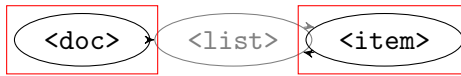
(c) The edge (&lt;list&gt;, &lt;item&gt;) is selected since the SCC containing &lt;item&gt; consists only of one node without a self-loop.
