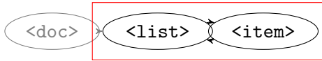
(b) The edge (&lt;doc&gt;, &lt;list&gt;) is not selected since the SCC containing &lt;list&gt; consists of two nodes.
