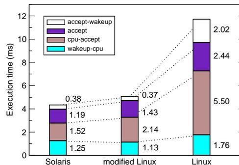
**Figure 10. The breakdown of the execution time of each thread in the thread pool in Linux with short time slices.**
