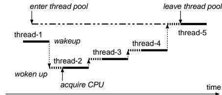
**Figure 5. The thread scheduling in the thread pool .**
