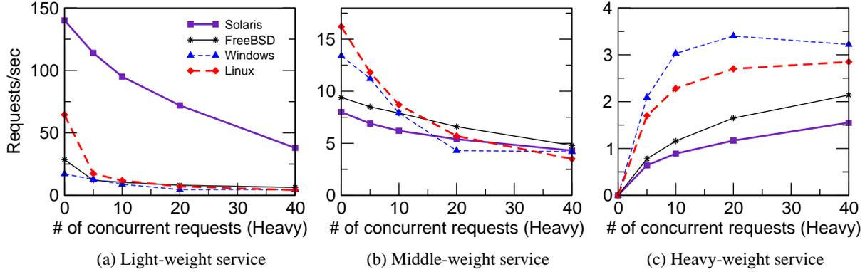
**Figure 3. The difference of degradation schemes among different operating systems for each service. (workload set 2)**
