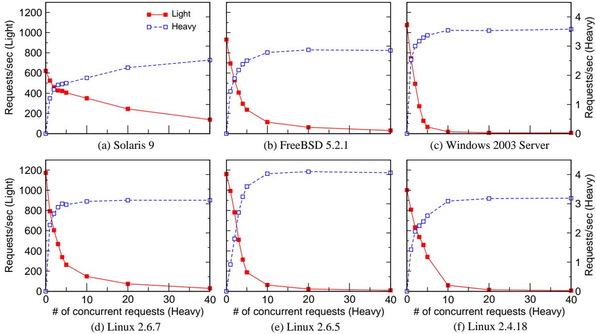
**Figure 1. Degradation schemes of various operating systems. (workload 1)**
