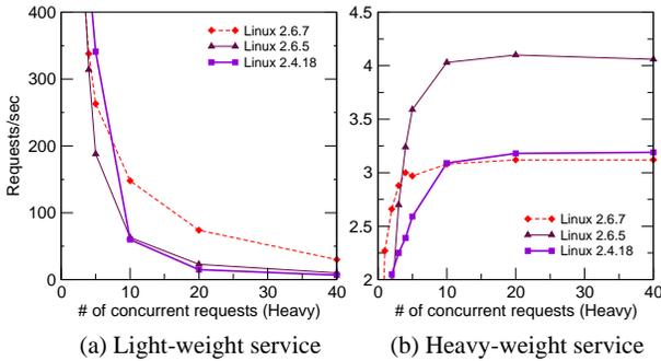
**Figure 4. The difference of degradation schemes among different versions of Linux for each service. (workload set 1)**
