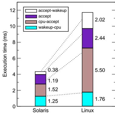
**Figure 6. The breakdown of the execution time of each thread in the thread pool (ms).**
