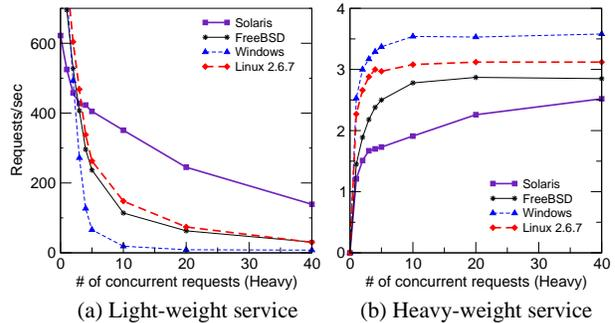
**Figure 2. The difference of degradation schemes among different operating systems for each service. (workload set 1)**
