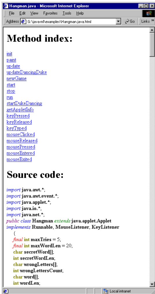
Figure 3: A view of Hangman.java.xml processed by an XSLT HTML pretty-printer and indexer. The method index links to the start of the definition of each method, and syntax highlighting is done using color-coding and italics.
